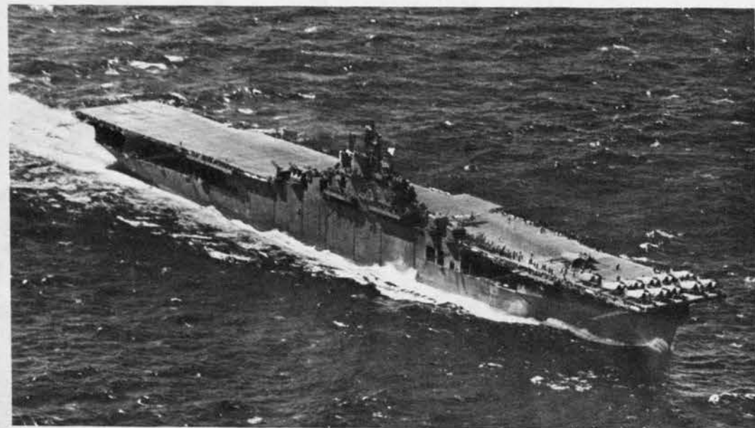
ESSEX'S ISLAND rises flush with hull almost directly amidships. The flight deck is square cut, with indentations forward and aft and a deck-edge elevator forming a projection opposite tower.
